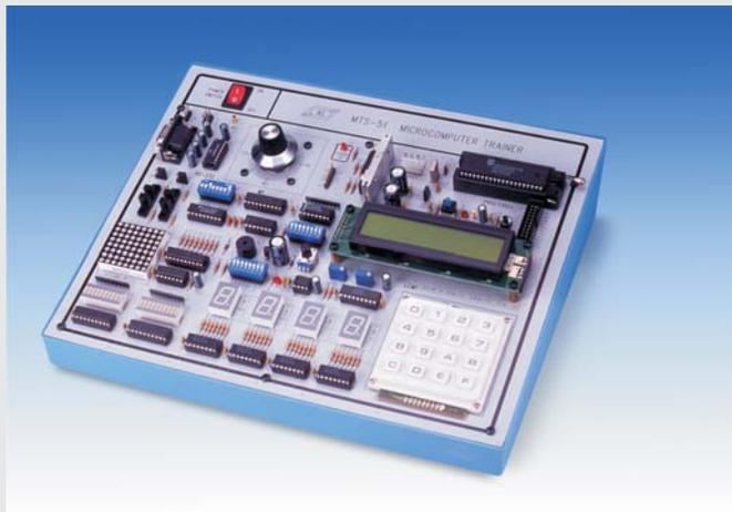
8051 is the original chip of MTS-51 family devices which is originated from Intel. This chip is a stand-alone, powerful 8-bit single-chip microcomputer and is commonly used for real-time control applications. MTS-51 microcomputer trainer is designed for learning 8051 core architecture and instructions.
