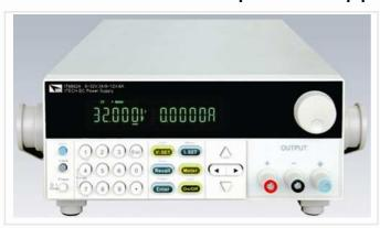
IT6860B power supply is a dual-range output power supply with high resolution of 1mV, 0.01mA, which can take place of two power supplies of previous type. You can adjust the voltage/current stepping by pressing the left and right keys to moving the cursor. It supports output timer function and programs by the front panel, which will bring great convenience. Its built-in RS232, USB and GPIB communication interfaces make the communication much faster.
